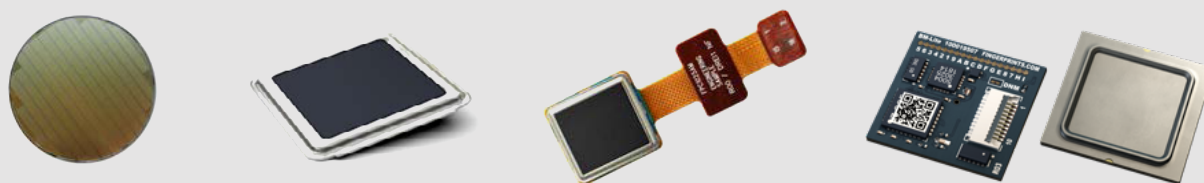
Figure 22. Wafer, LGA, module and stand-alone embedded system.
